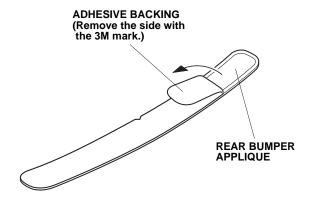
5. Spray the rear bumper applique with 3M protective tape application solution.
