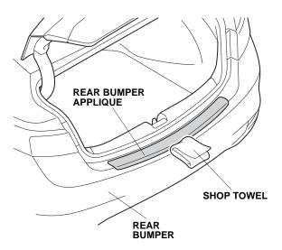
14. Remove the masking tape attached in step 2.
