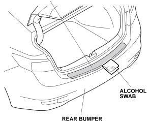
2. Attach a strip of masking tape to the rear bumper in the area shown. Using a felt-tip pen, make a mark on the tape at the center of the trunk lid anchor.
