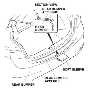
12. Use the soft sleeve to adhere the rear bumper applique to the lower section as shown.
