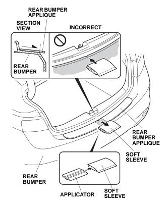
8. Starting from the center and working outward, use the soft sleeve to smooth out the center of the rear bumper applique upper section.
