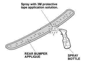
Align the v-notch on the rear bumper applique with the mark on the masking tape. Align the edge of the rear bumper applique with the bottom of the character line. Smooth the rear bumper applique against the rear bumper and the bottom of the character line.
